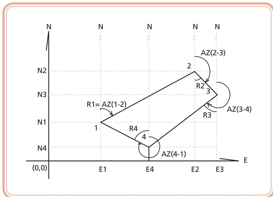
**Figura 3.10: Poligonal inserida no plano cartesiano com coordenadas UTM (E,N)**
